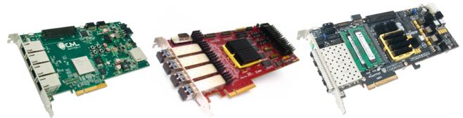
Figure 1: NetFPGA: the enabling platform of OSNT
