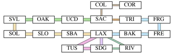
**Figure 1: CENIC hub sites are connected by an optical backbone. Long-haul fiber routes SVL to SAC, SVL to LAX, TRI to LAX, LAX–SDG, and LAX–TUS–SDG use the Cisco 15808 DWDM & 15454 platforms. Metro-area networks use a combination of CWDM and Cisco 15530 & 15540 DWDM equipment.**
